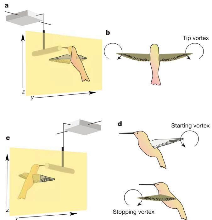
**Figure 1 | DPIV methodology.** **a**, Birds hovering at a feeder positioned such that the two-dimensional laser light sheet illuminated wake-entrained oil particles moving in a frontal plane. **b**, The expected wake structures within the frontal plane<sup>5,6</sup>. **c**, Light sheet oriented in the parasagittal plane, centred at midwing. **d**, The expected wake structures within the parasagittal plane<sup>5,6</sup>.
